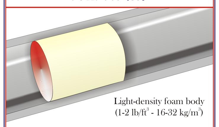
The Knapp Bare Swab Polly Pig offers the pipeline operator a pig with maximum flexibility that is able to negotiate extreme reductions in cross-sectional diameter as well as tight bends in pipelines. Available with a flat or a tapered nose, the Bare Swab is the most flexible Polly Pig that Knapp manufactures. The open-celled polyurethane foam body of the Bare Swab is extremely absorbent and is frequently used as a drying pig to help remove aby free water left after a pipeline dewatering project.
